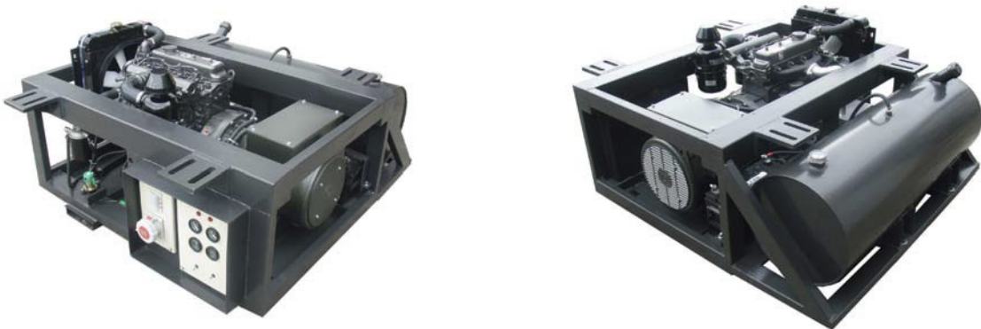
SCGC-3GL under-slung generator set inner structure
